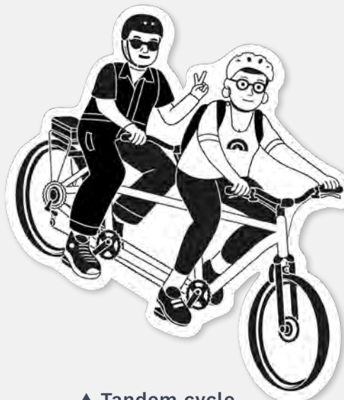
▲ Tandem cycle 0.65m (width) 2.4m (length), turning circle - 3.15m (Outer radius), 2.25m inner radius).
