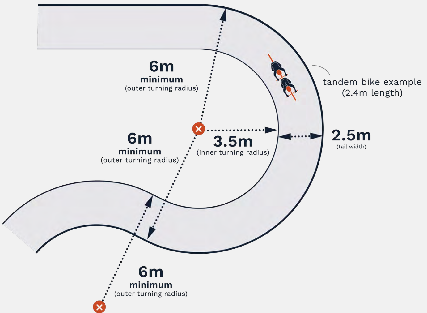
▲ Diagram 6: Turing radius — measuring a wide turning radius.
